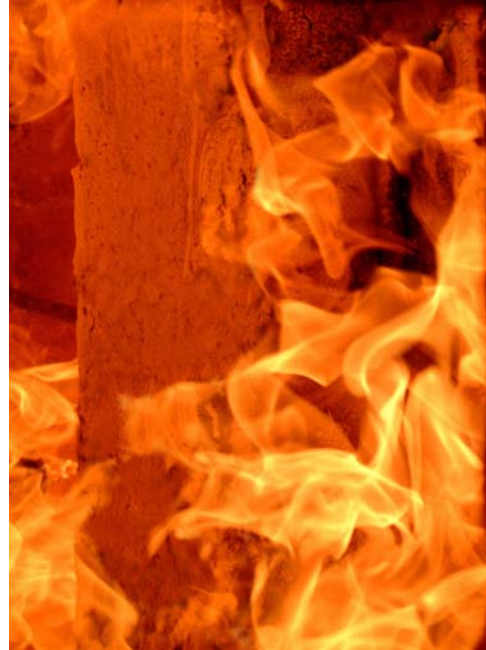
Figure 7-2 steel column with intumescent coating during fire test - Leighs Paint
