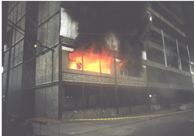
Figure 7-6 Cardington fire test - CORUS Steel
