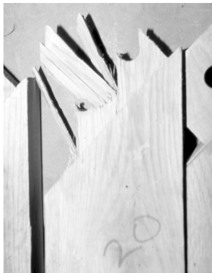
Figure 3-14 White Oak 2S2B Knee Brace Tenon Failure
