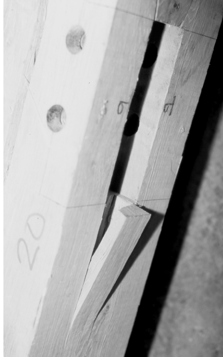
Figure 3-15 White Oak 2S2B Column Mortise Tear-out at Knee Brace Connection
