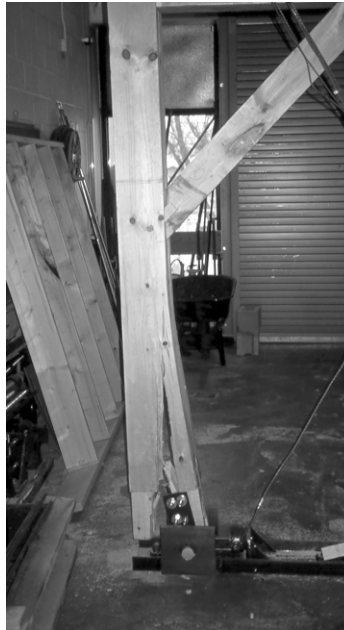
Figure 3-13 Eastern White Pine 2S2B Column Failure at Reaction
